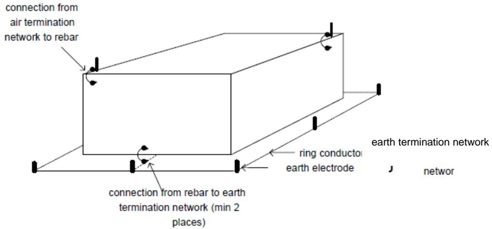
Figure C.1: Air termination network on a RC structure
