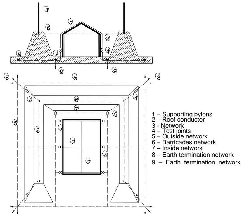
Figure C.10: The two levels of lightning protection systems
