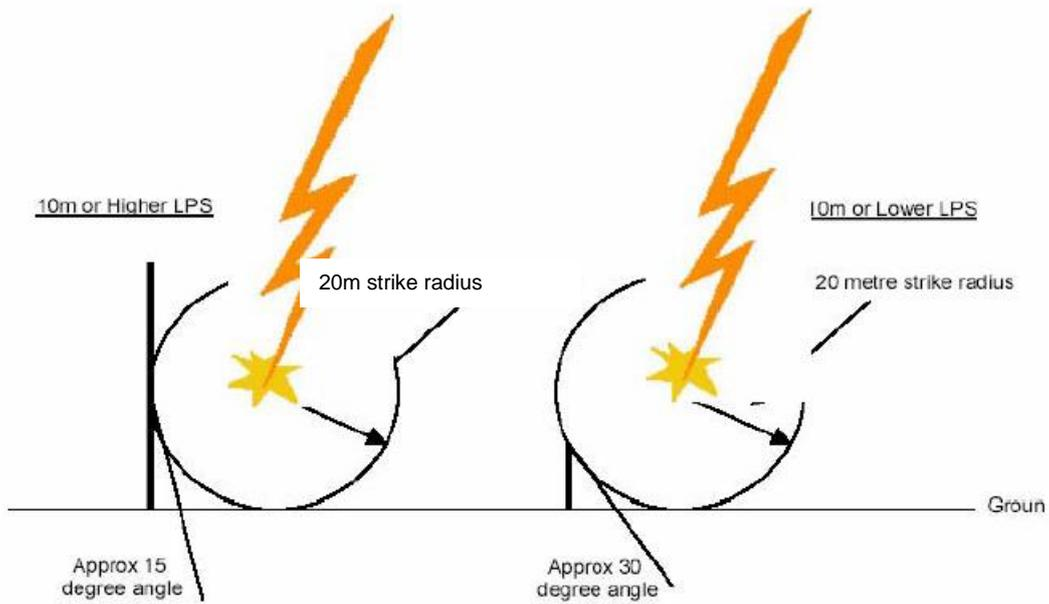
Figure C.9: The principle of the 20m rolling sphere
