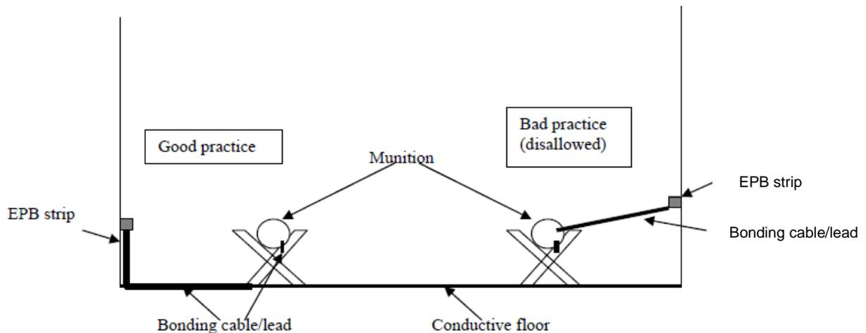
Figure 1: Bonding of ammunition with a connecting lead
