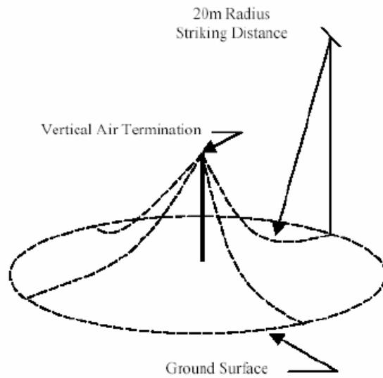
Figure C.7: Vertical air termination – 20m rolling sphere
