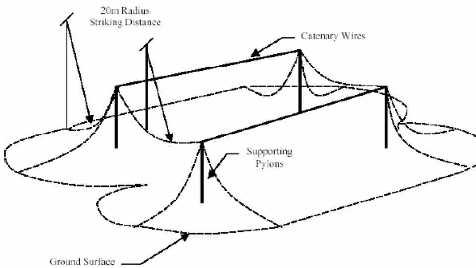
Figure C.8 Suspended air termination – 20m rolling sphere
