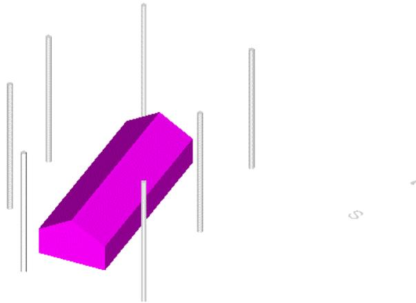
Figure C.11: Supporting pylons protection system around ammunition facility
