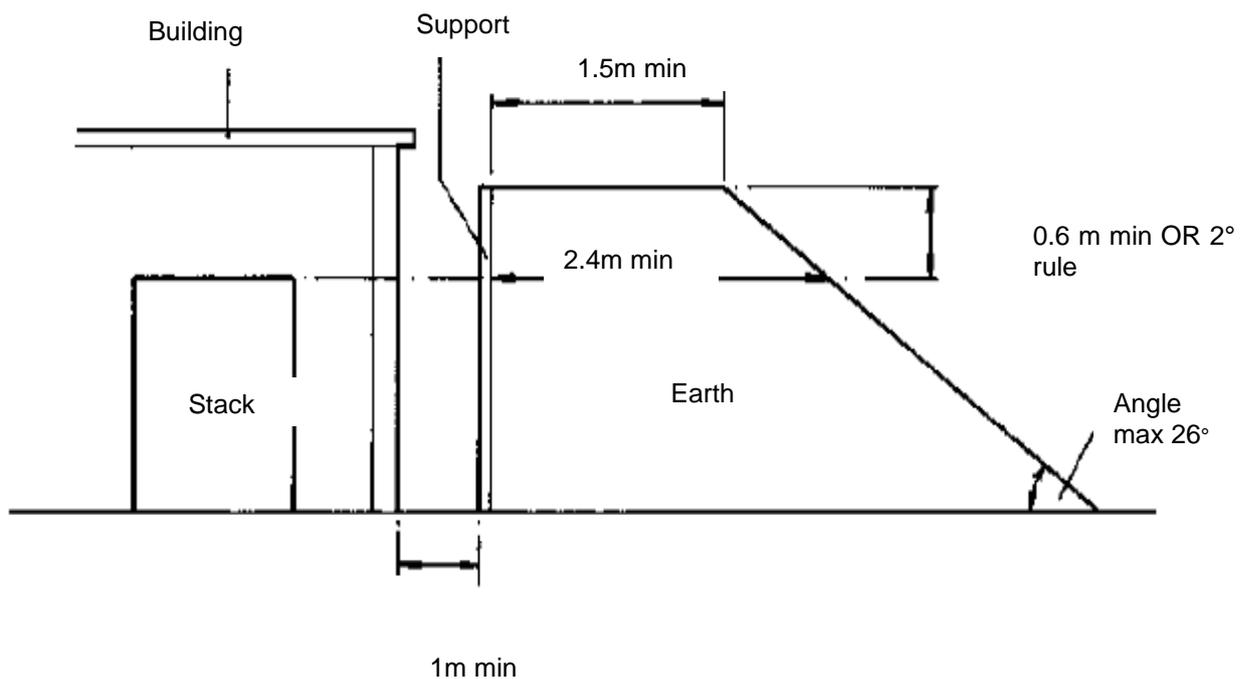
C.3 Type II – partly vertical partly sloped face type
