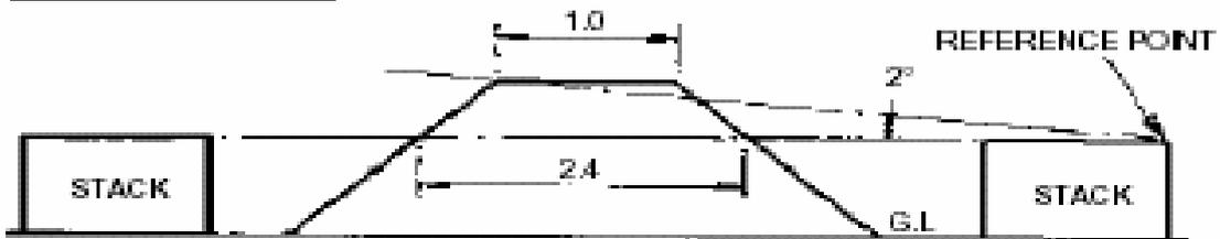
Fig 1 Determination of Traverse Height on Level Terrain
