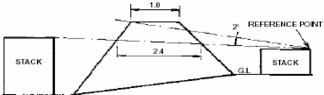
Fig 2 Determination of Traverse Height on Sloping Terrain
